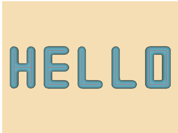
Figure 6.28: Implicit modelling used to thicken a stroked font. Original lines can be seen within the translucent implicit surface. ( Hello.cxx or Hello.py )
